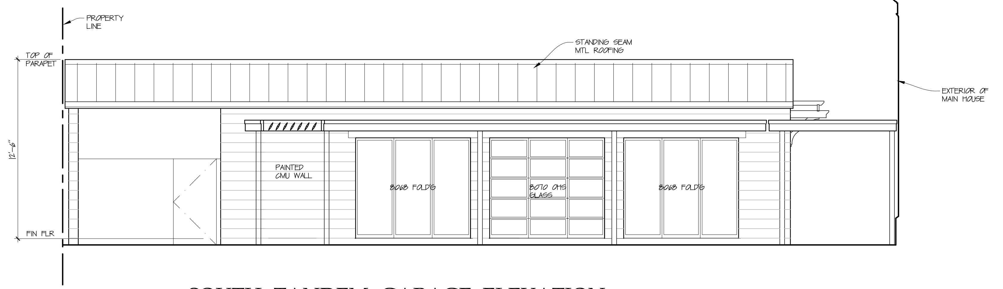
SOUTH TANDEM GARAGE ELEVATION SCALE: 1/4" = 1'-0" COURTYARD VIEW
